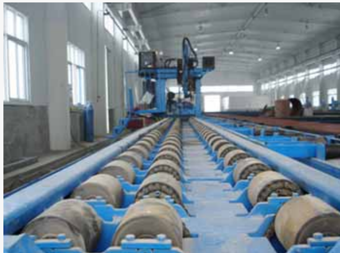
Pipe Bevel Machining Flow Line(B-type)
