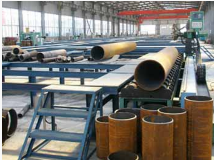
Pipe Bevel Machining Flow Line(B-type)
