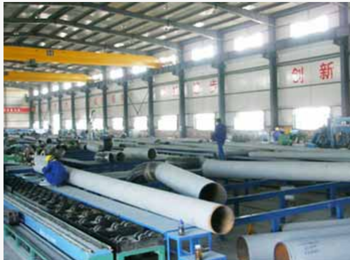
Pipe Bevel Machining Flow Line(B-type)
