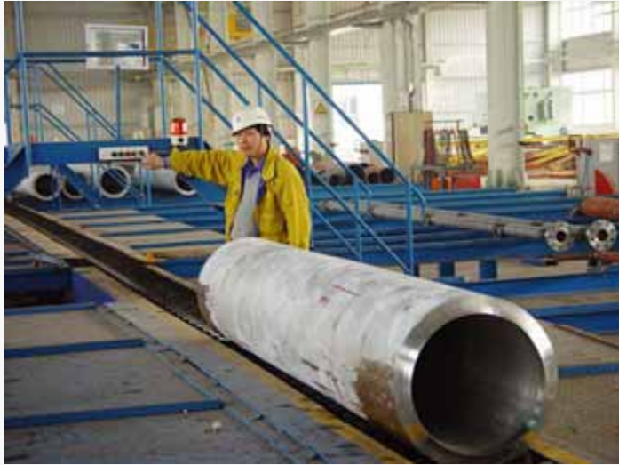
Pipe Logistics Automatic Transport System
