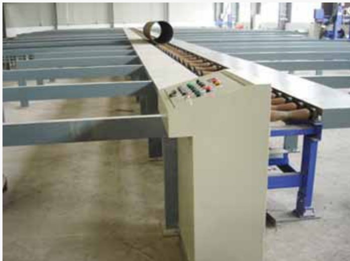
Pipe Logistics Automatic Transport System
