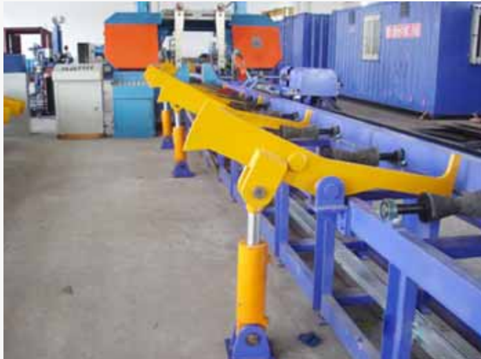
Pipe Logistics Transport System for Band Saw Machine
