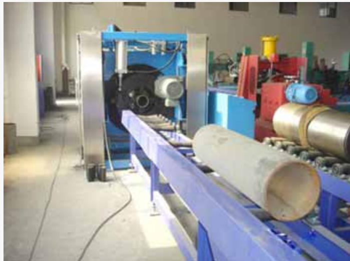
Pipe Logistics Transport System for Cutting and Beveling Machine
