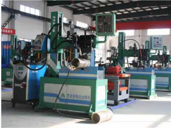
Piping Prefabrication Automatic Welding Machine(MIG)
