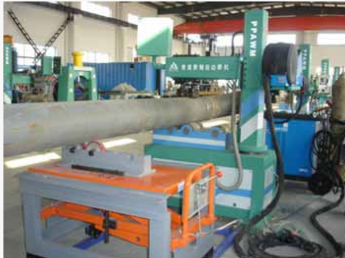
Piping Prefabrication Automatic Welding Machine(MIG)
