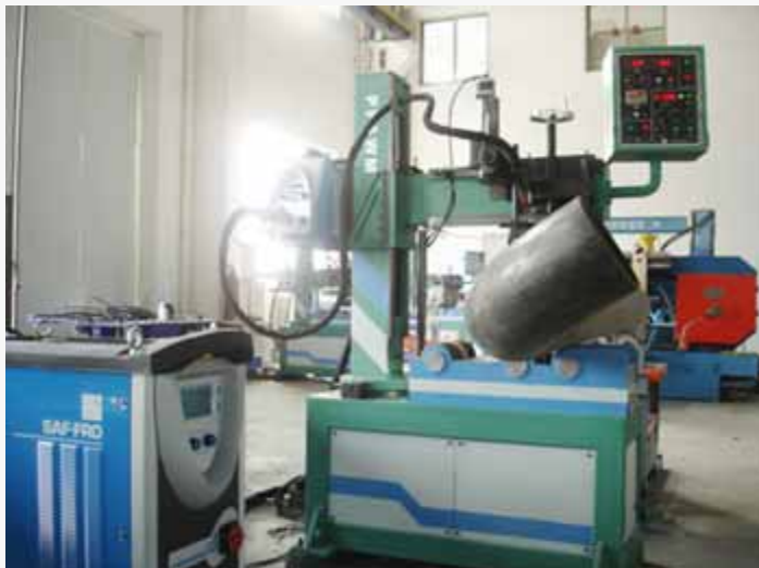
Piping Prefabrication Automatic Welding Machine(MIG)
