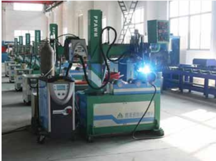
Piping Prefabrication Automatic Welding Machine(MIG)
