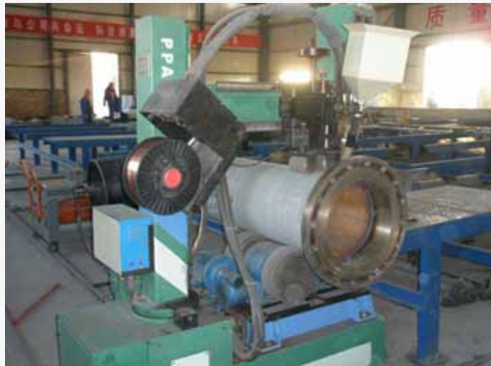
Piping Prefabrication Automatic Welding Machine(SAW)
