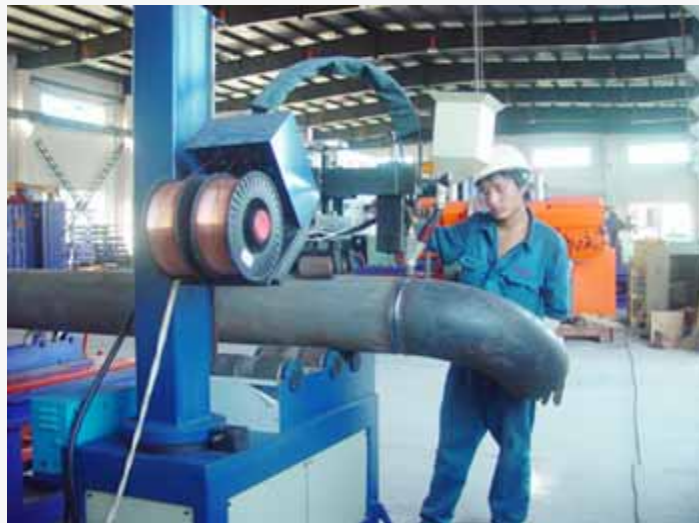
Piping Prefabrication Automatic Welding Machine(SAW)
