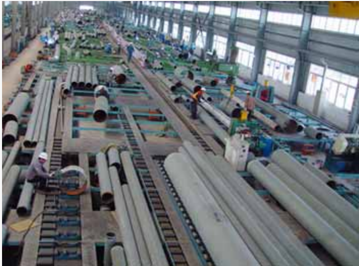
Piping Prefabrication Production Line (Fixed Type)
