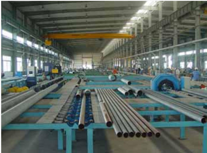
Piping Prefabrication Production Line (Fixed Type)
