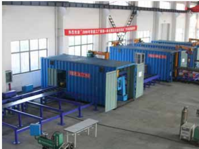
Tansportable Piping Prefabrication Production Line
