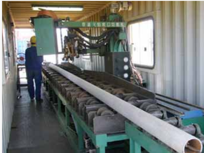
Transportable Piping Prefabrication Production Line
